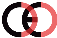
False CE Mark (too close)
