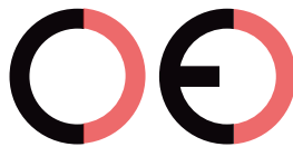
False CE Mark (too far)
