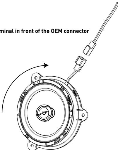
2 - Fix the speaker using the included rivets
